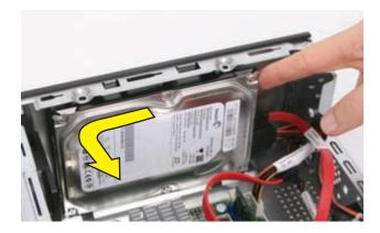
17 Lift the hard drive straight up and out.
